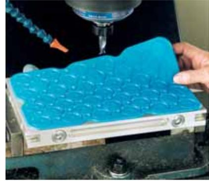
The lugs underneath the mat guarantee fast and accurate positioning of the VAC-MAT™ on the special modular vacuum chuck
