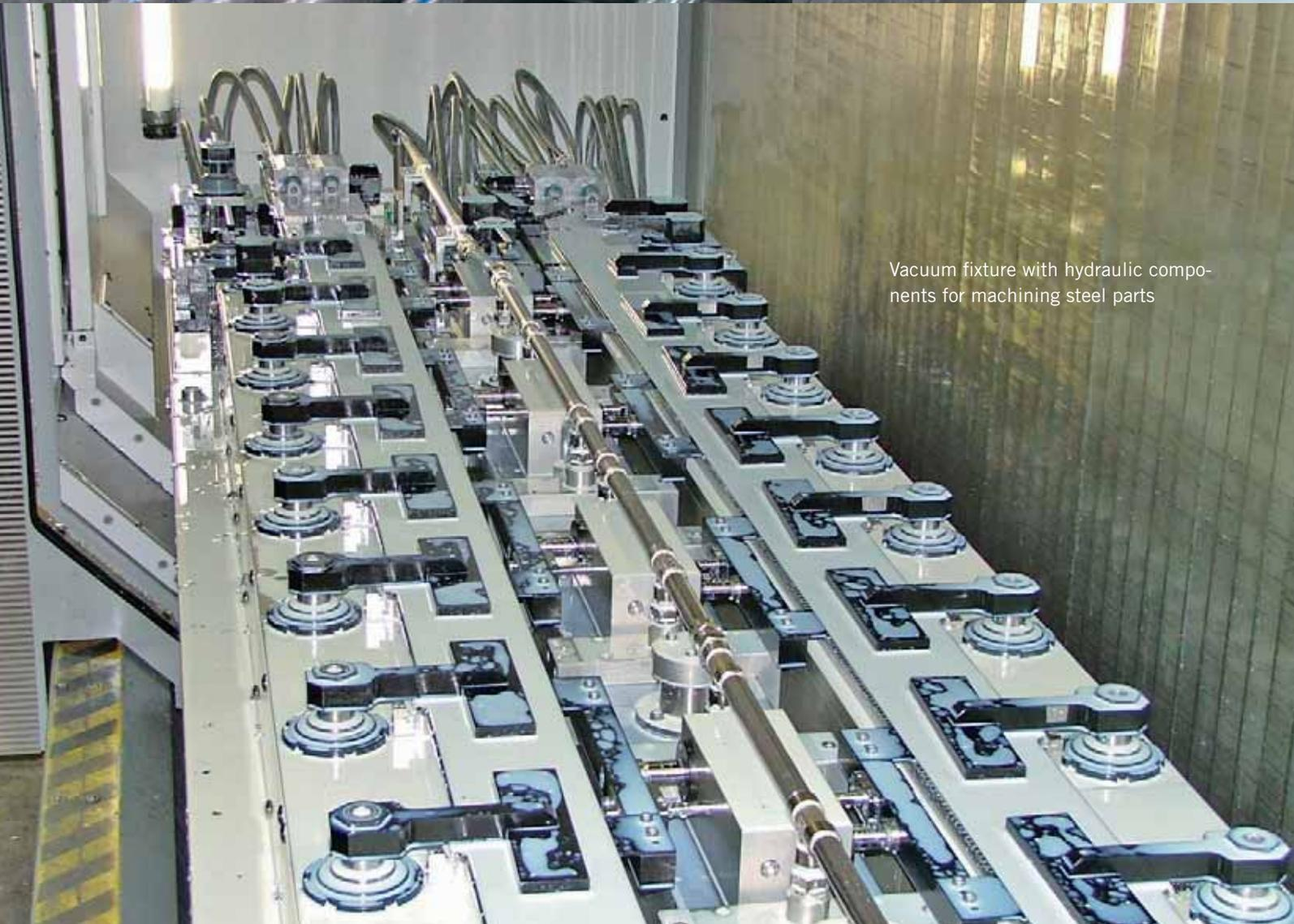
Vacuum fixture with hydraulic components for machining steel parts
