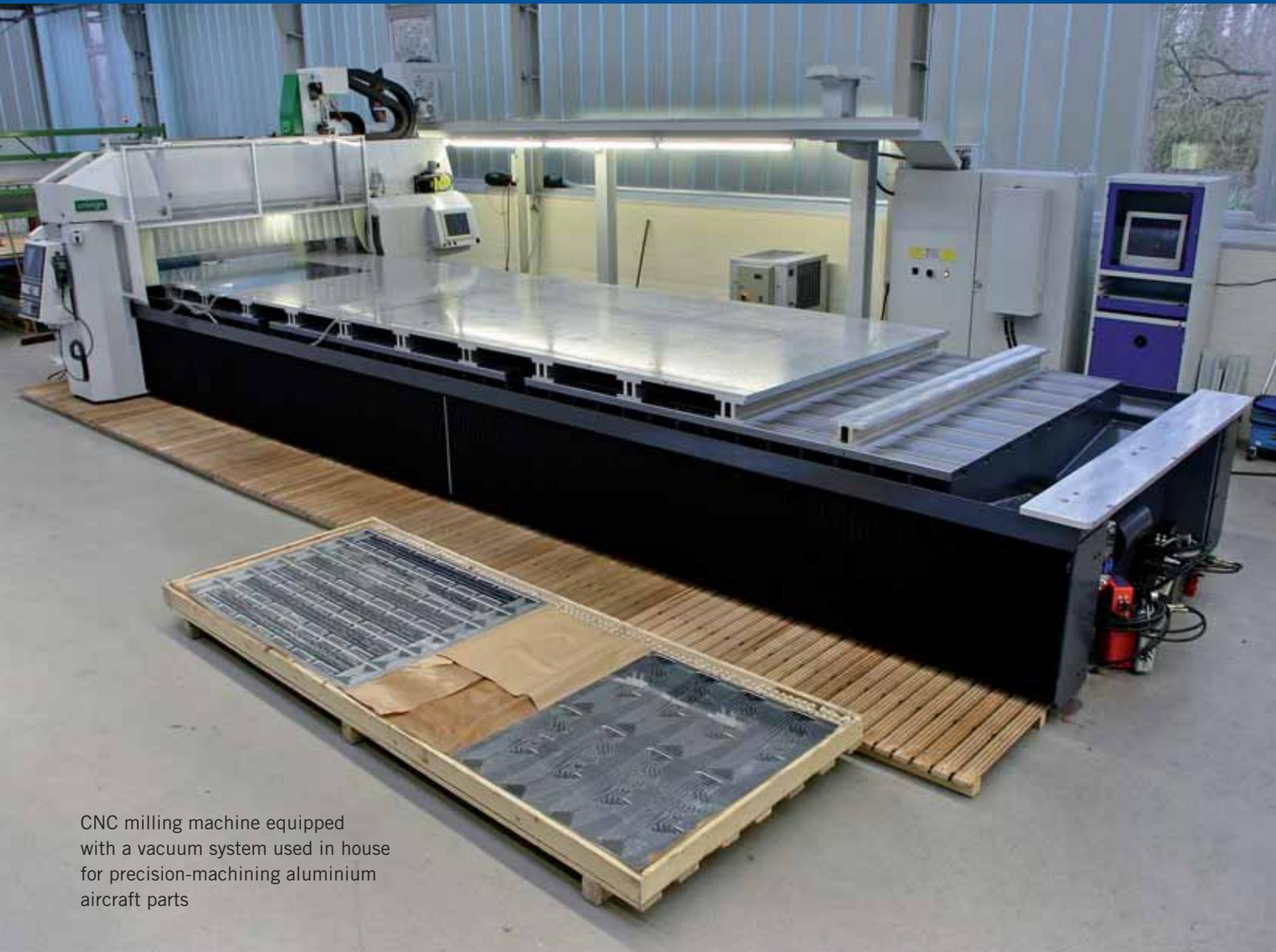
CNC milling machine equipped with a vacuum system used in house for precision-machining aluminium aircraft parts
