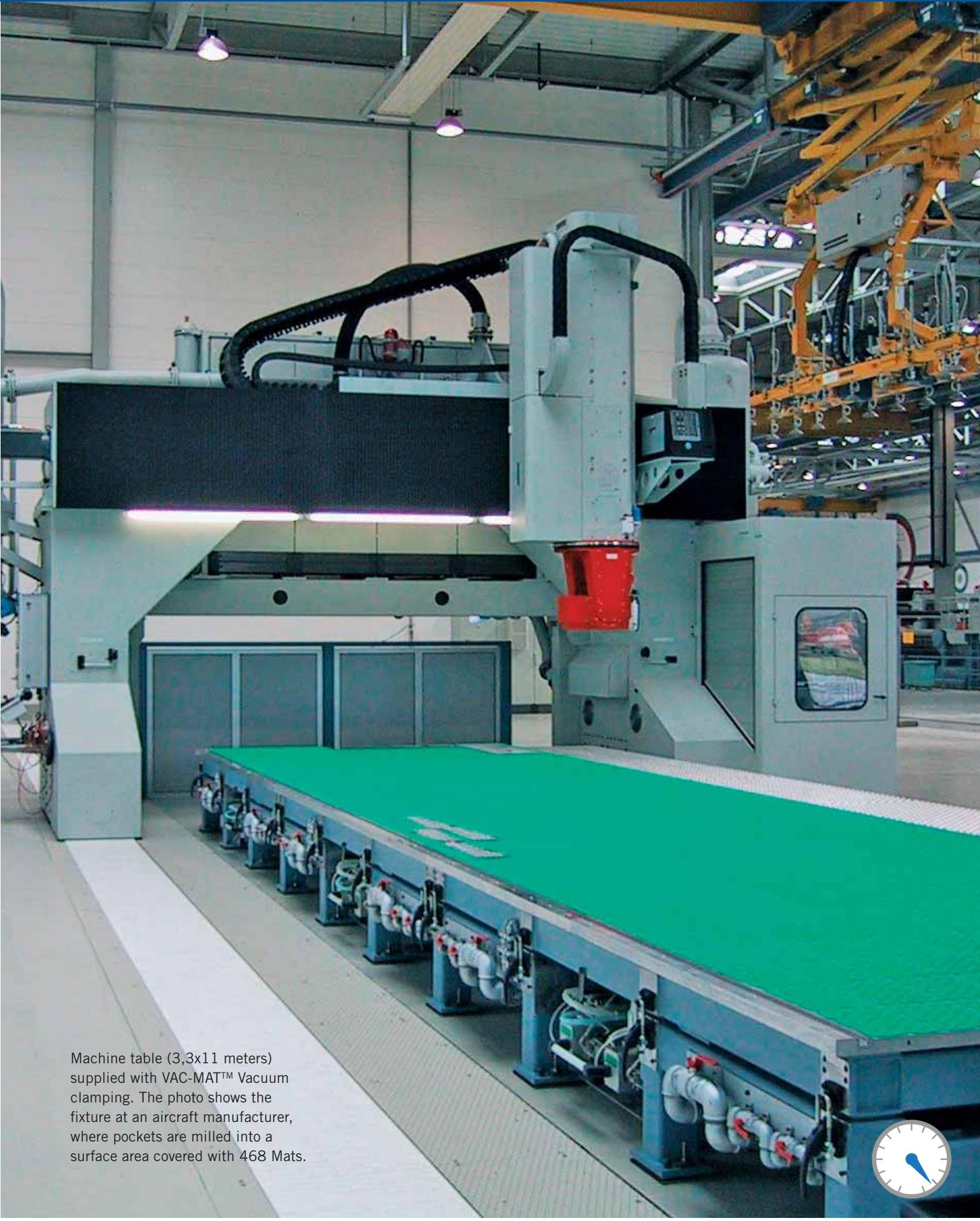
Machine table (3,3x11 meters) supplied with VAC-MAT™ Vacuum clamping. The photo shows the fixture at an aircraft manufacturer, where pockets are milled into a surface area covered with 468 Mats.
