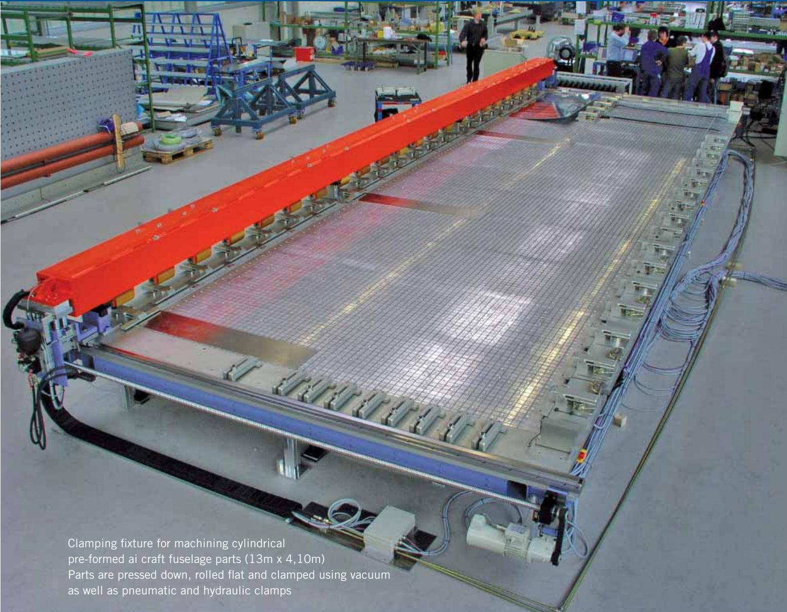
Clamping fixture for machining cylindrical pre-formed aircraft fuselage parts (13m x 4,10m)
