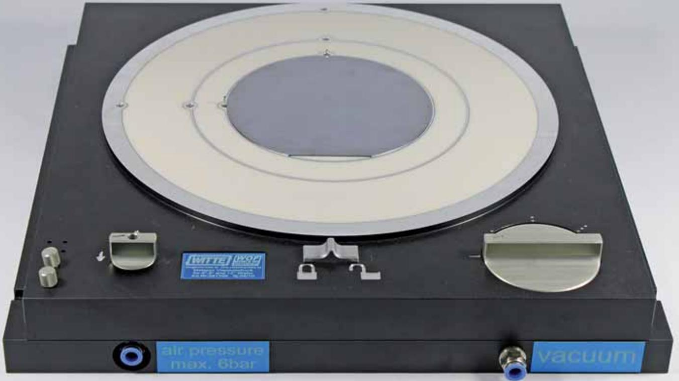
Specially designed porous chuck with three individual clamping areas, stops for part positioning and lifting pins for easy removal of wafers.
