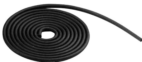
Used for sealing grid chucks or defining active vacuum areas. This high quality seal is placed into the slot of a grid type vacuum chuck.
