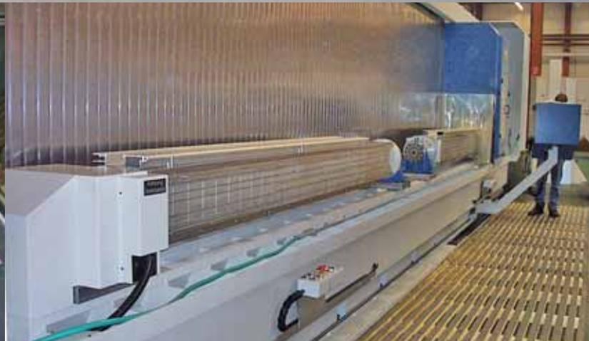
2 Rotating systems (each 3500mm) with vacuum clamping areas on all four sides for machining aluminium profiles
