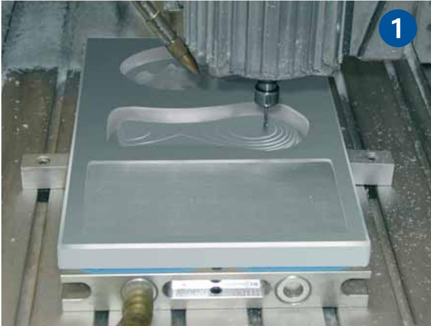
Left: First step is milling workpiece conventionally
