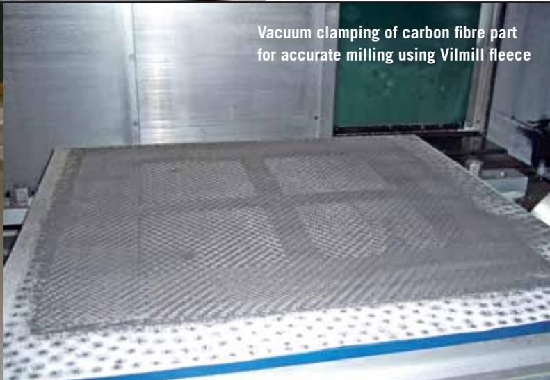
Vacuum clamping of carbon fibre part for accurate milling using Vilmill fleece
