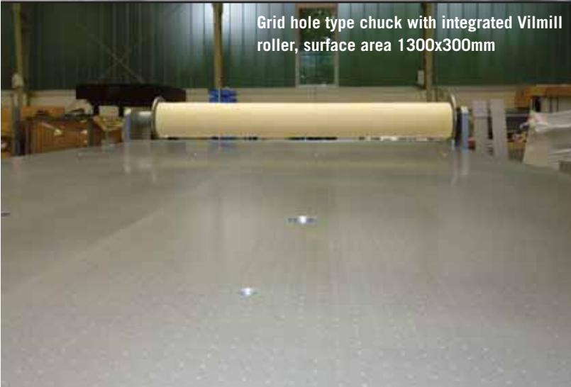
Grid hole type chuck with integrated Vilmill roller, surface area 1300x300mm
