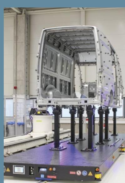
Structure plates from the Witte FixBase® range are ideally suited as a base for column type fixture design.
