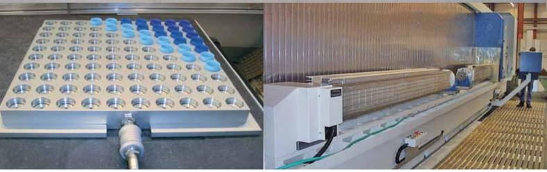
Vacuum chuck for clamping bottles tops during measuring by coordinate measuring machine
