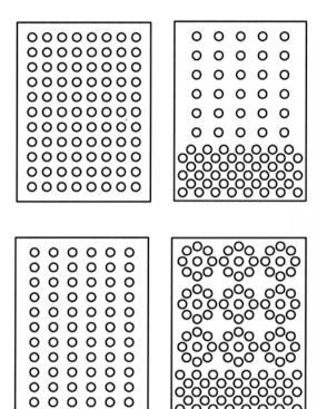
The user can choose a panel design that best suits the parts being machined. The pod panel can be laid out in almost any design and combination.
