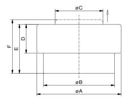
Acts as spacer when positioning large workpieces, raised ring retracts when vacuum is applied
