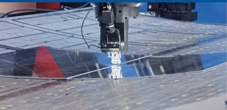
3D Vacuum chuck with several movable segments for clamping aircraft fuselage parts during milling and friction stir welding processes
