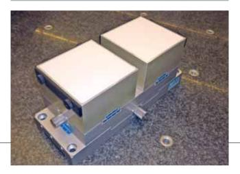
Double chuck system with two clamping surfaces which can be very accurately aligned to one another
