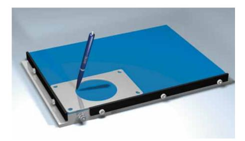
Using the slot chuck with the rubber adapter mat allows drilling of holes and milling or cutting of pockets and cutouts into the mat to a depth of 1,5mm without losing vacuum. As the mat suffers hardly any wear and tear it can be used often for workpieces with the same contour.
