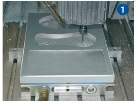
Left: First step is milling workpiece conventionally
