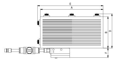
1. Vacuum generation simply by using compressed air on site: The built-in vacuum pump (Venturi system) requires operating pressure of 4-6 bar.
