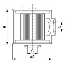
Universally used dust filter, dirt immediately visible through transparent housing. Designed to allow easy exchange of cartridge, whereby filter seals must also be changed. A fitting filter cartridge is included in package.
