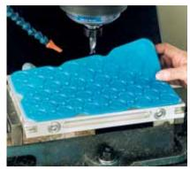
The lugs underneath the mat guarantee fast and accurate positioning of the VAC-MAT<sup>™</sup> on the special modular vacuum chuck
