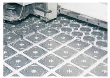
Machining of aluminum sheets of greater thickness
