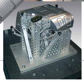
Vacuum fixture for clamping aircraft wing parts during friction-stir welding
