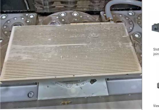
Slot vacuum chuck mounted on a zero reference clamping system
