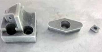
When clamping with the lce-Vice system parts are frozen to chuck surface on a capillary film of water for machining. Even relatively uneven parts can be clamped as any gaps are filled with water. The vertical and horizontal clamping forces created are enough to hold small parts for milling, grinding, drilling or polishing.
