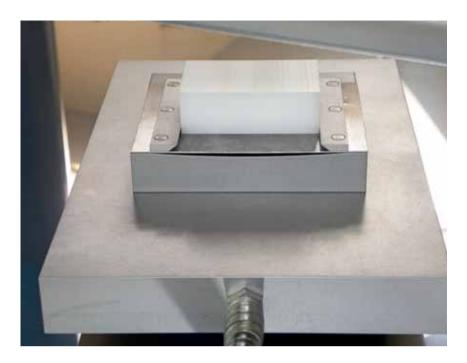
For example, if on a milling center several consecutive processes require re-clamping of a part and the remaining surfaces for direct vacuum clamping are too small, this innovative clamping technology can be used.
